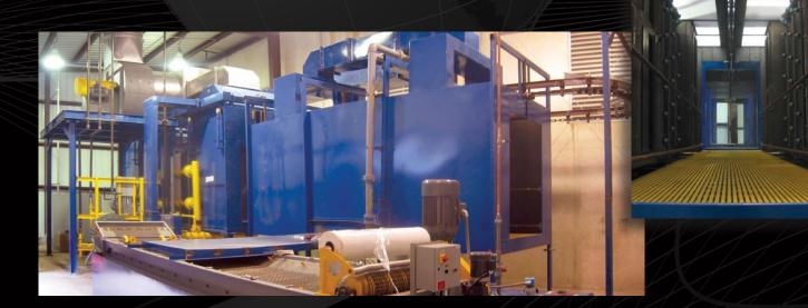
Speed, efficiency and cost savings make the GFS Process Heater, Rapid Heat Transfer (RHT) the smart choice for high-volume rack stripping applications. In as little as four to six minutes, the RHT removes paint from racks and hooks. The secret to it's amazing performance is high velocity manifolds and rapid heat transfer technology. Plus, the remarkable dual-pass in-line system which also means less energy usage, lower costs, and more available floor space.
