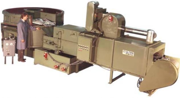
**POST PROCESS CONVEYOR SYSTEMS** like our two stage wash / dry conveyor above can be added to your SVB Series Bowl Machine. Ask for Wash/Dry literature for details.
